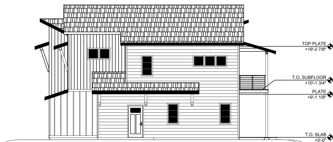
RIGHT SIDE ELEVATION BUILDING A
